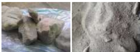
Figure 3. lump of waste silica sand (left) and crushed sand (right)
